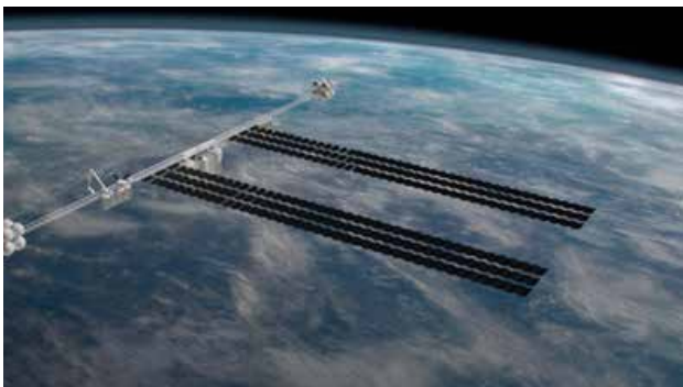
Satellites with solar panels would need to be around 1.7km long - more than double the size of the world's tallest building and an order of magnitude bigger than the current largest structure in space, which is the International Space Station, measuring 110m
