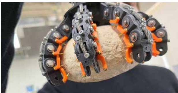
The inspiration for this robot claw came from the way tarantulas grip on to walls
