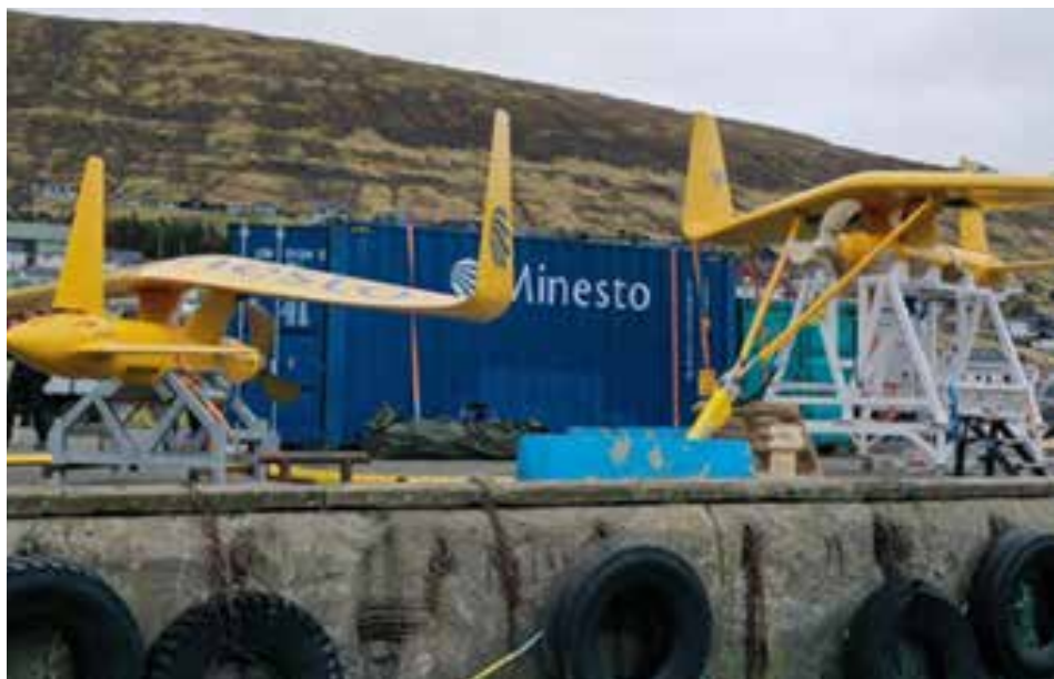
The energy-generating kites "fly" under the water, tethered to the seabed
