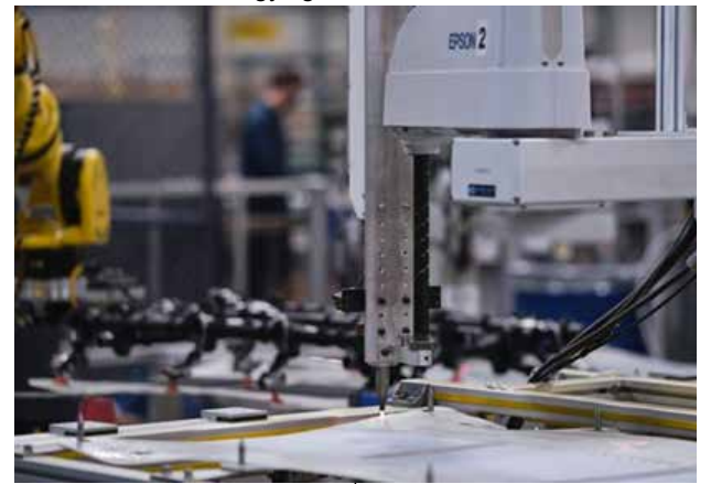
Plastic sheets are treated with plasma at the ESS manufacturing facility in Wilsonville, Oregon
