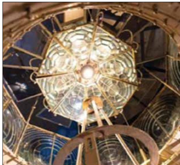
By arranging a series of small prisms into the shape of a beehive, Augustin Fresnel discovered he could capture and refract oblique light
