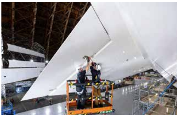
Pathfinder 1 has tail fins at an angle because aerodynamic knowledge is much more refined than in the 1930s
