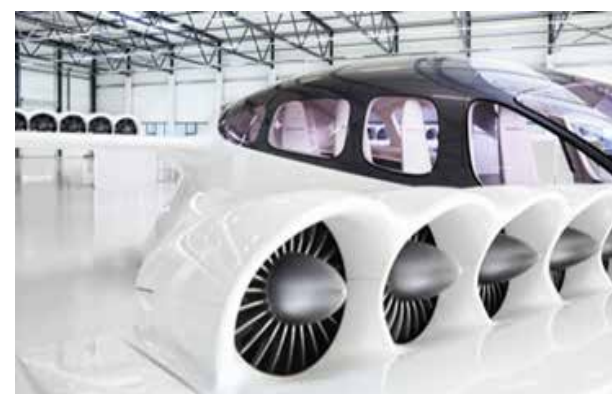
The Lillium EVTOL uses electric jets which swivel between take-off and forward flight
