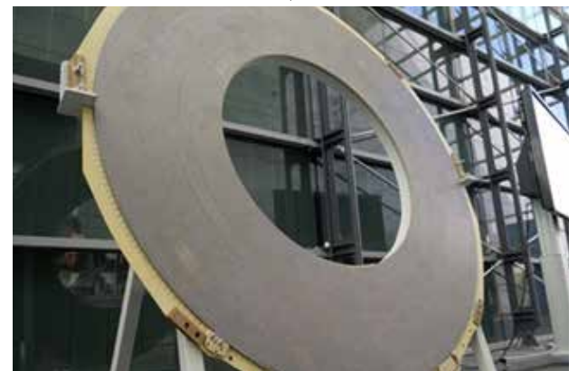
Just one of the superconductor coils used to form a giant magnet for the world's most powerful MRI scanner
