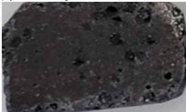
A picture of the purported superconducting material LK-99. Pic: Sukbae Lee, Ji-Hoon Kim, Young-Wan Kwon
